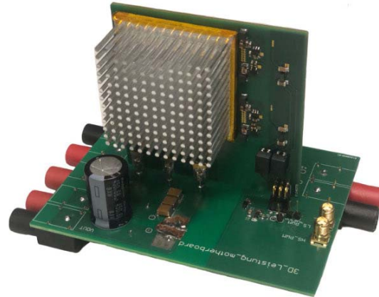
Figure 3.50: The double pulse test platform based on half-bridge topology
