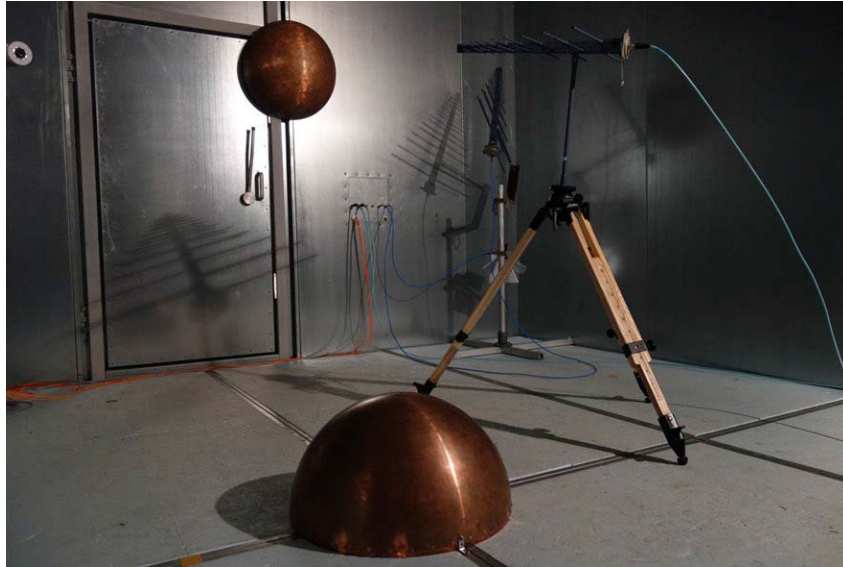
Figure 3.42: Measurement setup with copper hemispheres on the wall and the floor of a reverberation chamber with dimensions of 5.3 \text{ m} \times 3.7 \text{ m} \times 3 \text{ m}
